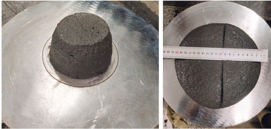
FIGURE 3: Fluidity test of graphite concrete.
