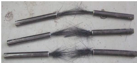
FIGURE 3: Rupture of CFRP tendon.
