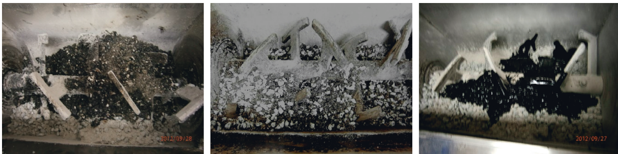
FIGURE 2: Step 2—addition of RA, step 3—addition of virgin binder [2].
