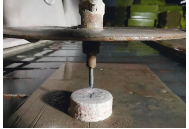
FIGURE 2: Pre-crack preparation in CSCFBD specimens using a water jet cutting machine [4].
