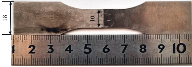
FIGURE 19: The shape and dimensions of the welded samples.
