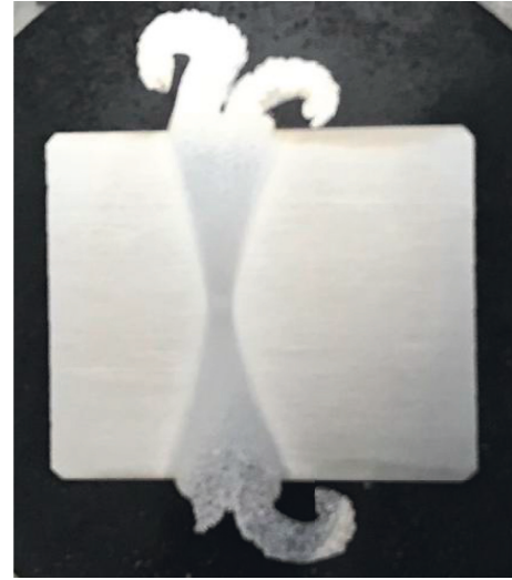
FIGURE 11: Typical microstructure of a rotary friction weld in Ti6Al4V.
