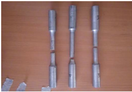
FIGURE 3: Test specimen (after test).
