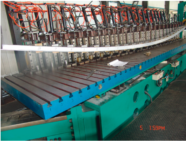
FIGURE 8: The detection setup and the forming part through the MPSB process.
