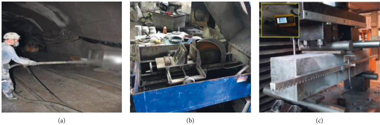
FIGURE 1: Beam specimen preparation: (a) underground concrete shot and curing, (b) slab cutting, and (c) beam specimen with a crack detector.
