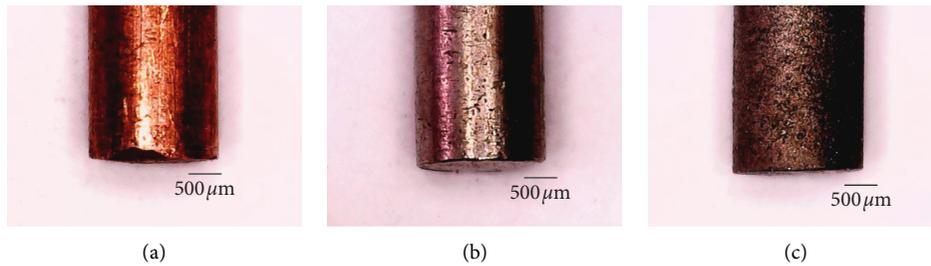
FIGURE 3: Composite tools. (a) Common copper tool. (b) Nickel-coated tool. (c) Diamond-nickel-coated tool.
