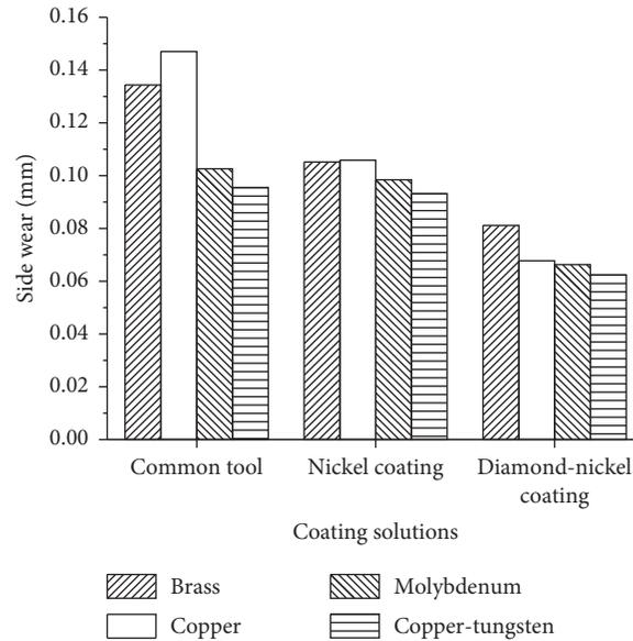
FIGURE 10: Side wear of different coated tools.
