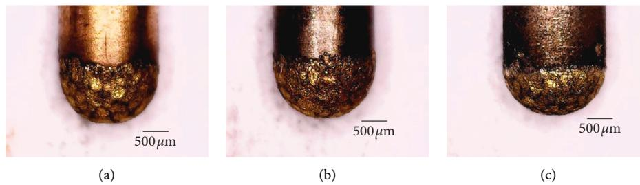
FIGURE 11: Shape change of brass-based composite tools. (a) Common tool. (b) Nickel-coated tool. (c) Diamond-nickel-coated tool.
