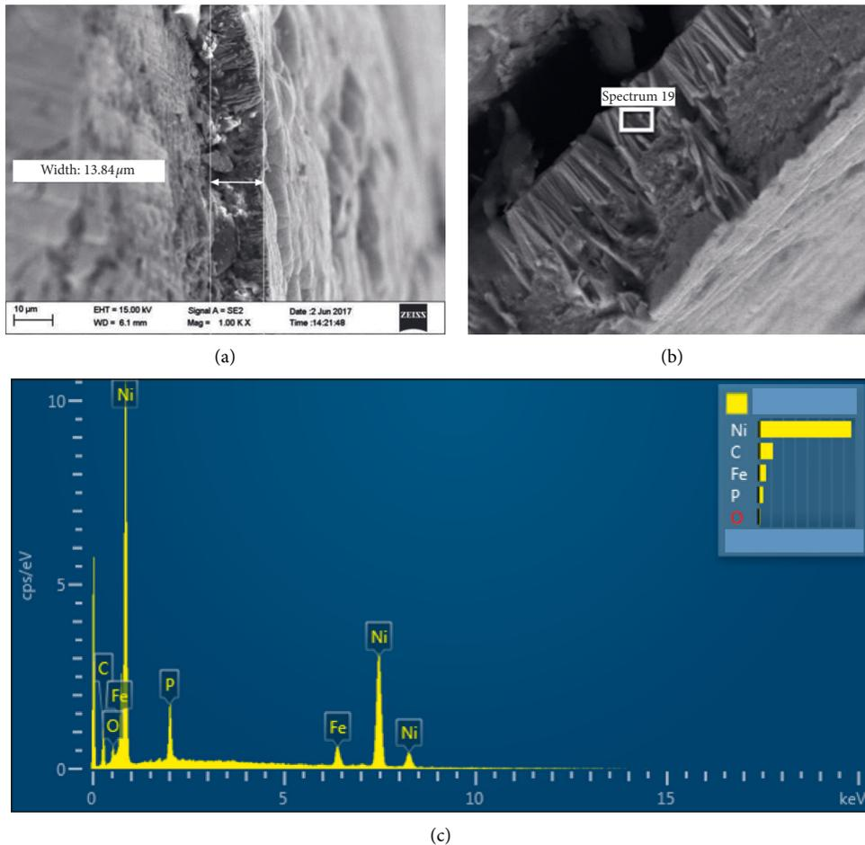
FIGURE 4: SEM image of the copper tool with nickel coating. (a) Thickness image of the composite tool. (b) Local image of the composite tool. (c) Local energy spectrum analysis of the copper tool.
