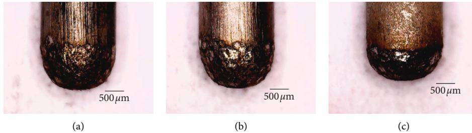
FIGURE 8: Shape changes of molybdenum composite tools. (a) Common tool. (b) Nickel-coated composite tool. (c) Diamond-nickel-coated composite tool.
