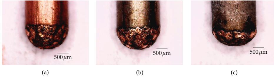
FIGURE 7: Shape change of copper-based composite tools. (a) Common tool. (b) Nickel-coated tool. (c) Diamond-nickel-coated tool.
