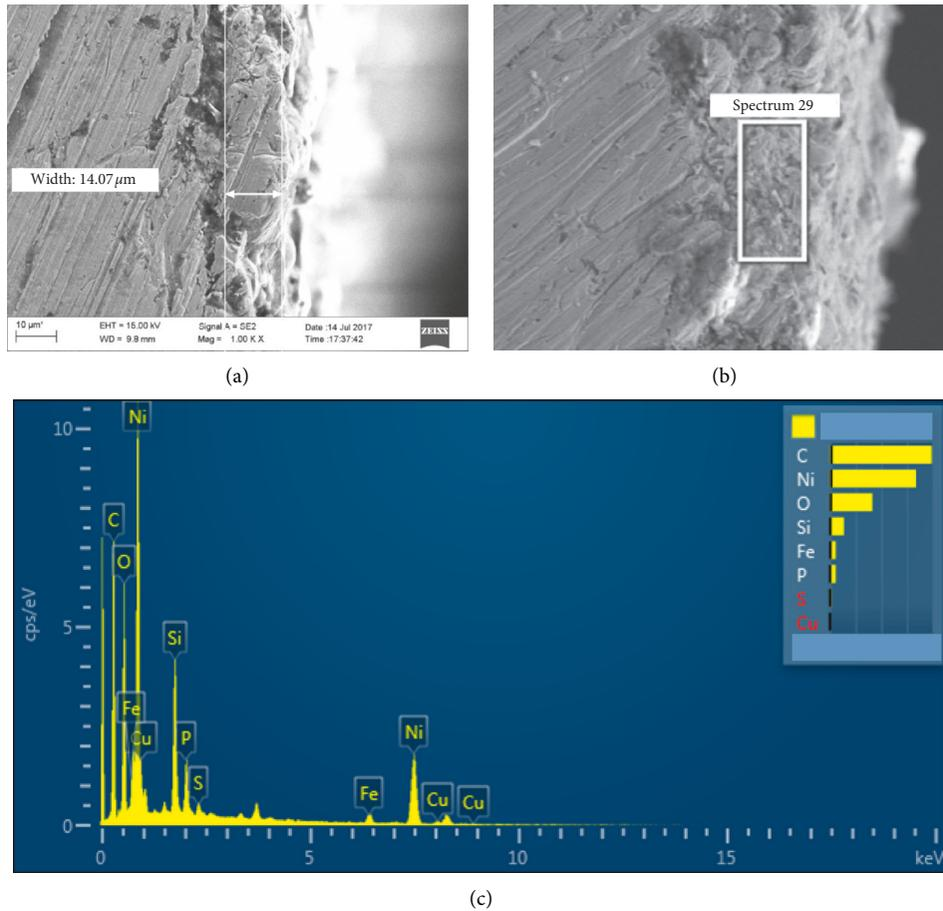
FIGURE 5: SEM image of the copper tool with diamond-nickel coating. (a) Thickness image of the composite tool. (b) Local image of the composite tool. (c) Local energy spectrum analysis of the copper tool.
