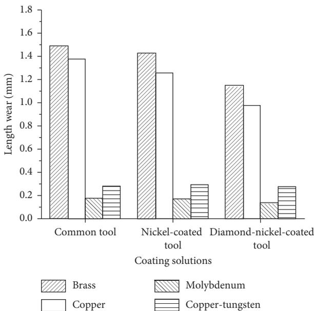
FIGURE 6: Length wear of different coated tools.
