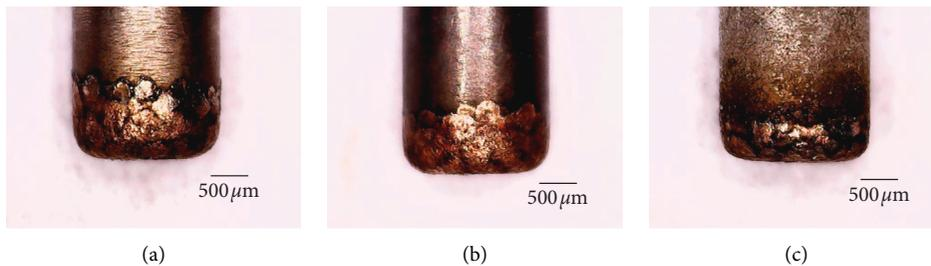
FIGURE 9: Shape changes of copper-tungsten alloy composite tools. (a) Common tool. (b) Nickel-coated composite tool. (c) Diamond-nickel-coated composite tool.
