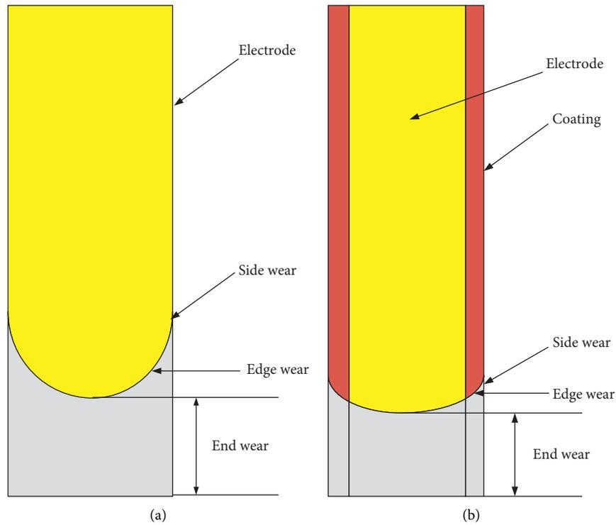
FIGURE 1: Comparison of (a) common tool wear and (b) coated tool wear.
