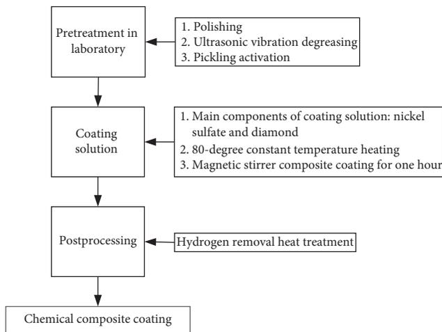
FIGURE 2: Chemical composite coating flow chart.
