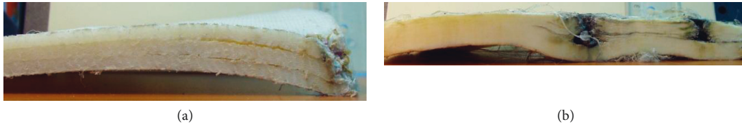
FIGURE 12: (a) Cross-sectional view of 3 plies of composite structures after impact; (b) Cross-sectional view of the laminated composite structure after impact.
