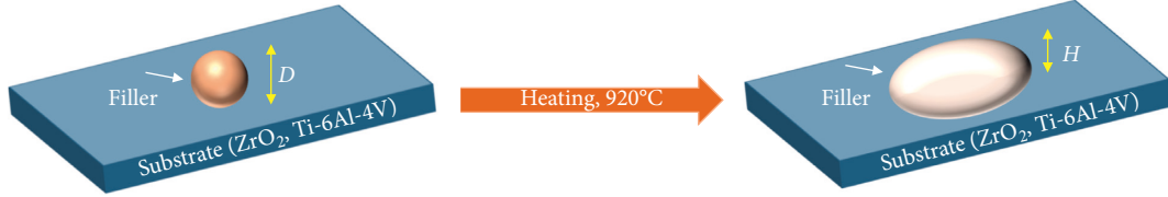
FIGURE 1: Schematic diagram for the measurement of brazeability.
