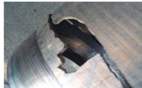
FIGURE 19: Spinning fracture defect.
