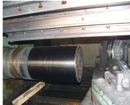
FIGURE 15: Hot rotary core mold installation state.
