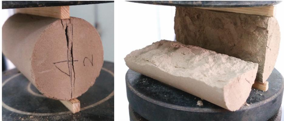
FIGURE 3: Indirect tension test.
