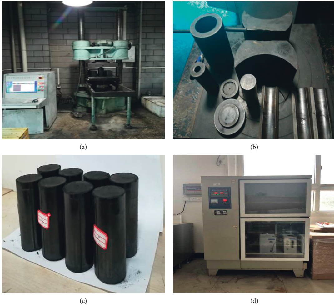
FIGURE 2: (a) Forming equipment, (b) moulds, (c) moulded coal, and (d) curing box.
