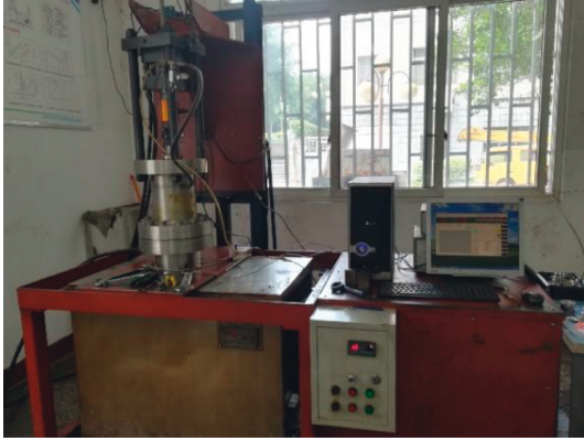
FIGURE 1: Triaxial servo-controlled seepage equipment for hot-fluid-solid coupling of coal containing methane.
