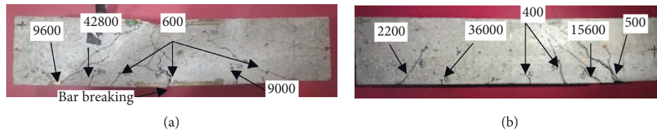
FIGURE 8: Fatigue failure mode of test beams. (a) Normal cross section failure. (b) Oblique section failure. Number in the fatigue means the number of cycles when each crack started to initiate.
