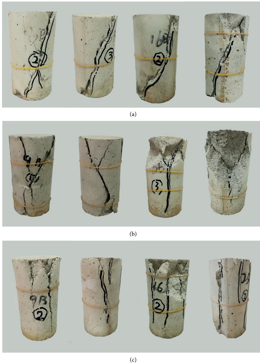
FIGURE 10: Three types of typical failure modes of uniaxial compression tests: (a) shear failure of single inclined plane; (b) Y-shaped tensile shear failure; (c) pure tensile failure.
