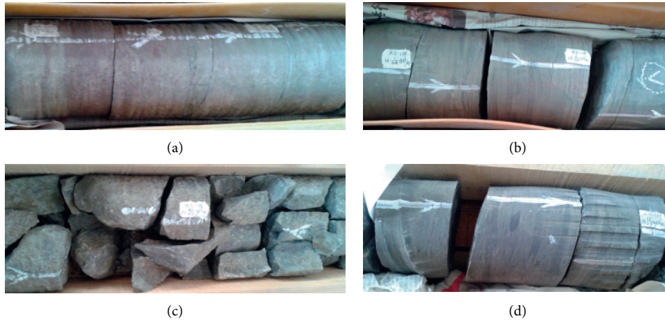
FIGURE 1: Origin rocks drilled from D5-1 well: (a) argillaceous siltstone, depth of 2315.7 m~2320.9 m; (b) mudstone, depth of 2327.3 m~2331.7 m; (c) mudstone, depth of 2331.7 m~2339.9 m; (d) mudstone, depth of 2339.9 m~2342.6 m.
