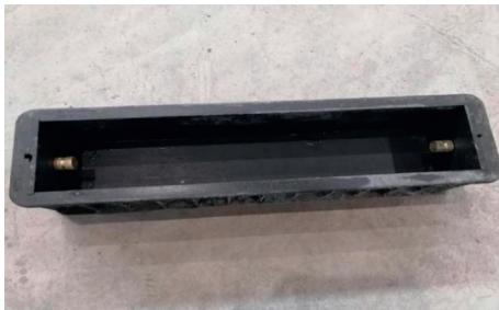
FIGURE 1: Concrete shrinkage test block mould.
