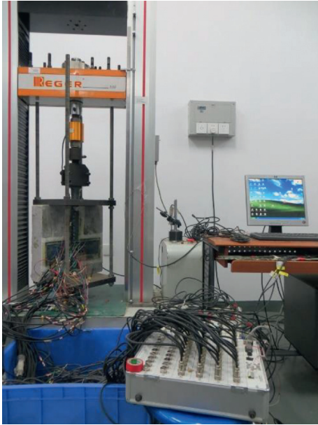
FIGURE 2: Test setup for single shear test.
