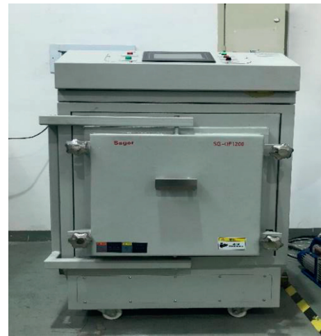
FIGURE 5: Box-type atmosphere furnace.
