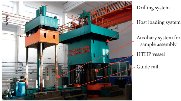
FIGURE 1: 600°C 20 MN servo-controlled triaxial rock mechanics testing machine.
