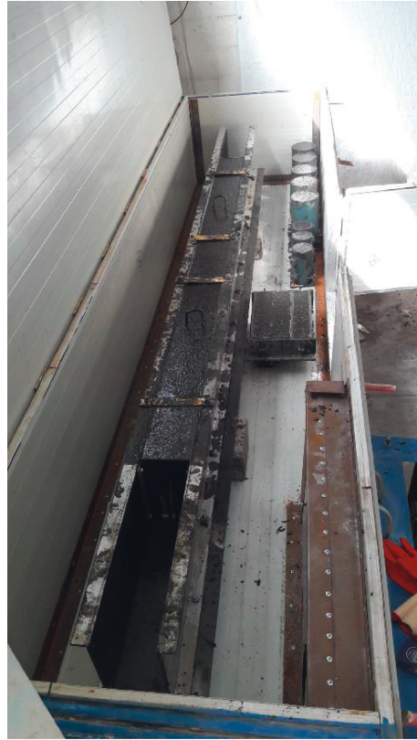
FIGURE 3: Casted beam specimen inside the oven.
