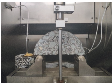
FIGURE 9: Photograph of the assembly of semicircular split samples.
