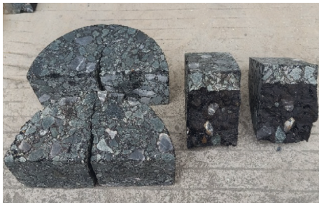
FIGURE 8: Photograph of the failed semicircular split samples.
