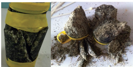
FIGURE 5: Macroscopic damage mode of granite.
