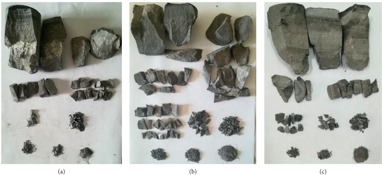
FIGURE 7: Sieving results of limestone fragments obtained under the uniaxial stress state. (a) Conventional compression test. (b) Cyclic loading test with a frequency of 0.25 Hz. (c) Cyclic loading test with a frequency of 0.5 Hz.
