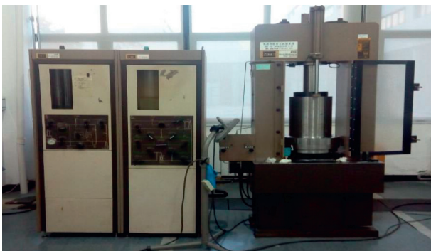
FIGURE 3: MTS815.02 rock mechanics test system.
