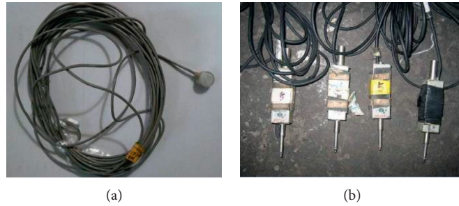
FIGURE 5: Test sensor. (a) Miniature pressure box; (b) displacement sensor.
