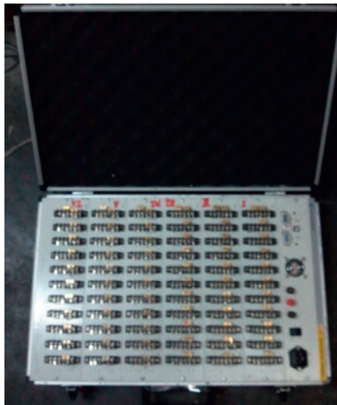
FIGURE 6: Static strain gauge.
