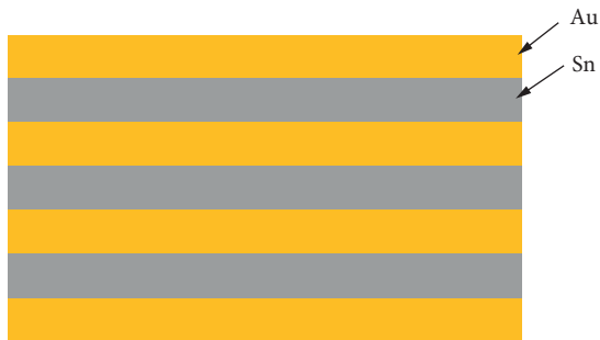
FIGURE 15: Gold-tin laminated soldering diagram.
