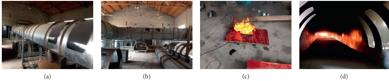
FIGURE 8: (a) Model of tunnel. (b) Model of cross channel. (c) Testing the heat release rate of fire source. (d) Testing the smoke diffusion when a fire occurs in a two-lane tunnel.
