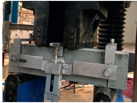
FIGURE 3: Bending toughness test device.
