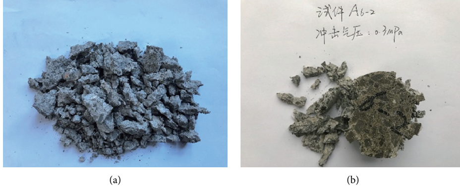
FIGURE 8: The failure pattern of specimens under 0.3 MPa: (a) A1; (b) A6.
