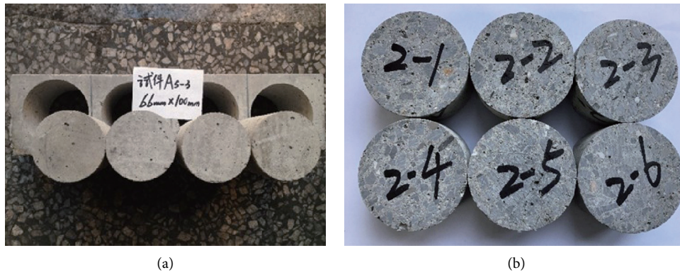
FIGURE 2: Specimens for SHPB tests: (a) after coring; (b) after cutting and grinding.
