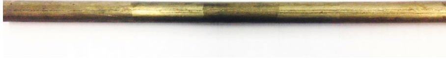
FIGURE 1: CuAlMn SMA bar with a bamboo-like grain structure.
