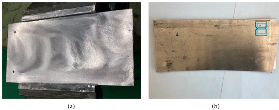
FIGURE 7: The Al-Ti-Al laminated plate. (a) Before rolling. (b) After rolling.
