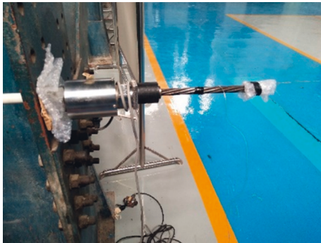
FIGURE 6: Diagram of anchorage, gaskets, and pressure sensor.
