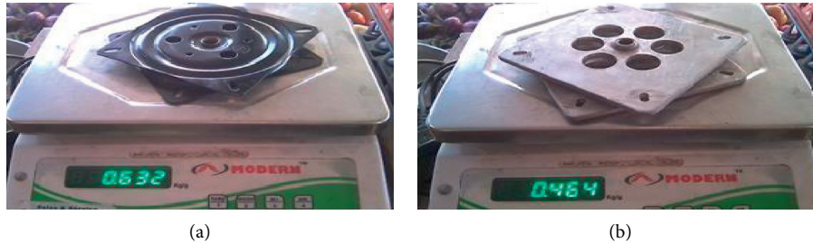
FIGURE 16: Weight difference between Mg alloy and A3 steel swivel plate. (a) Weight of A3 steel swivel plate. (b) Weight of Mg alloy swivel plate.
