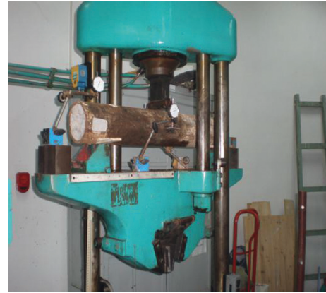
FIGURE 9: The simply supported bending test.
