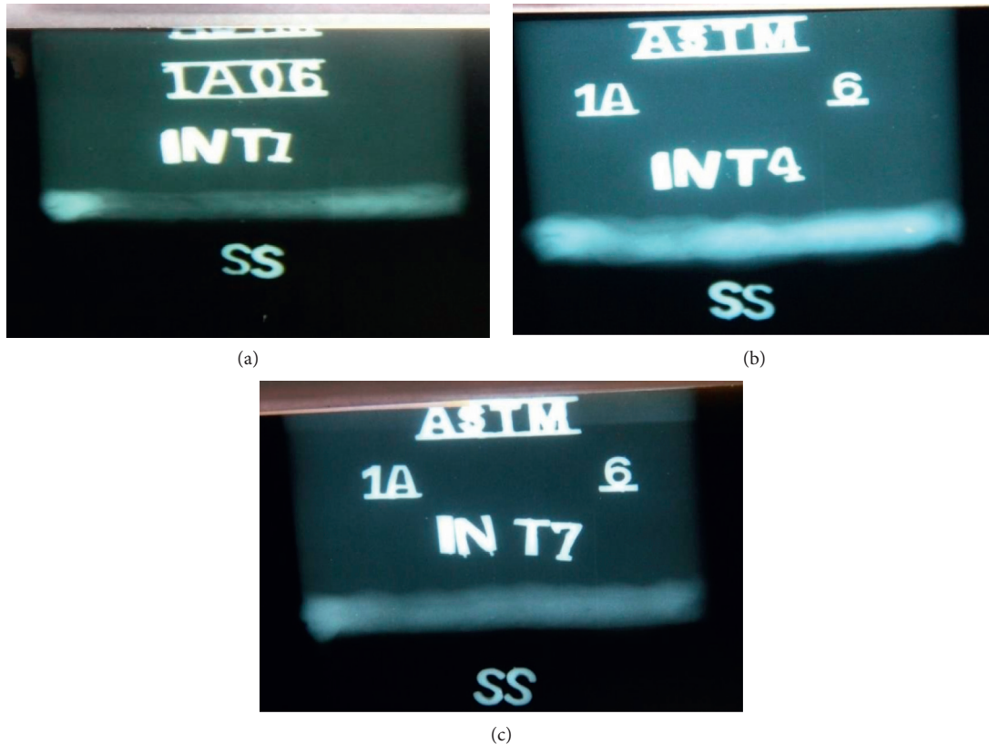
FIGURE 4: Radiography test of the weldments.
