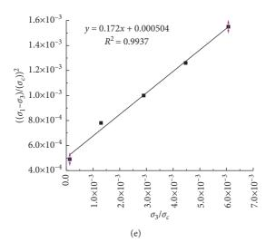
FIGURE 7: Determination of empirical parameters m and s for each sample. Empirical parameters m and s of (a) sample I, (b) sample II, (c) sample III, (d) sample IV, and (e) sample V.
