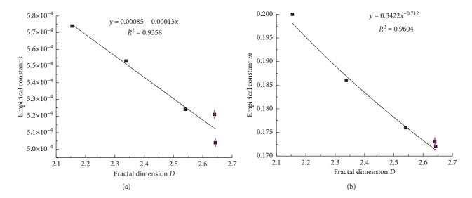
FIGURE 8: Fractal dimension and empirical parameter relation curve of extremely fractured phyllite at fault fracture zone. (a) Relationship between fractal dimension D and s of extremely fractured phyllite. (b) Relationship between fractal dimension D and m of extremely fractured phyllite.
