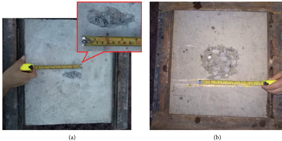
FIGURE 13: Test results of the cylindrical explosive. (a) Upper surface. (b) Bottom surface.
