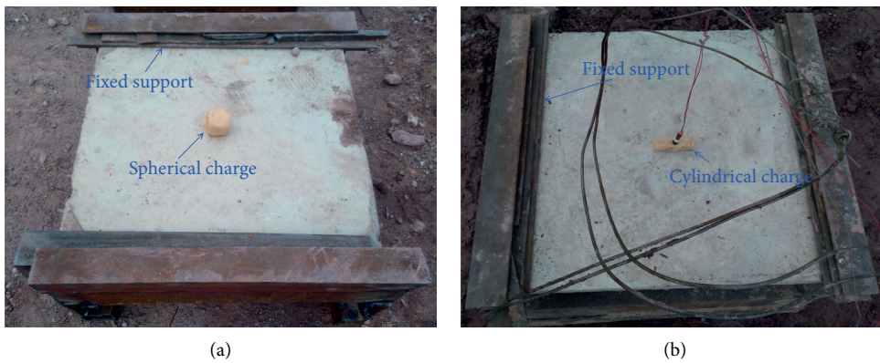
FIGURE 11: Air contact blast tests setup. (a) Spherical explosive. (b) Cylindrical explosive.
