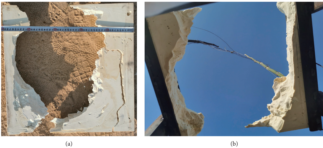
FIGURE 14: Test results of polymer slab B3 under 30 g explosive. (a) Top surface. (b) Bottom surface.
