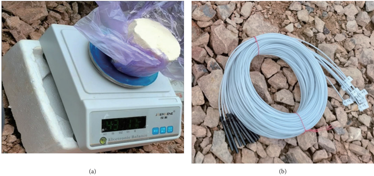
FIGURE 3: Explosive charge and detonator. (a) Rock emulsion explosive. (b) Detonator.
