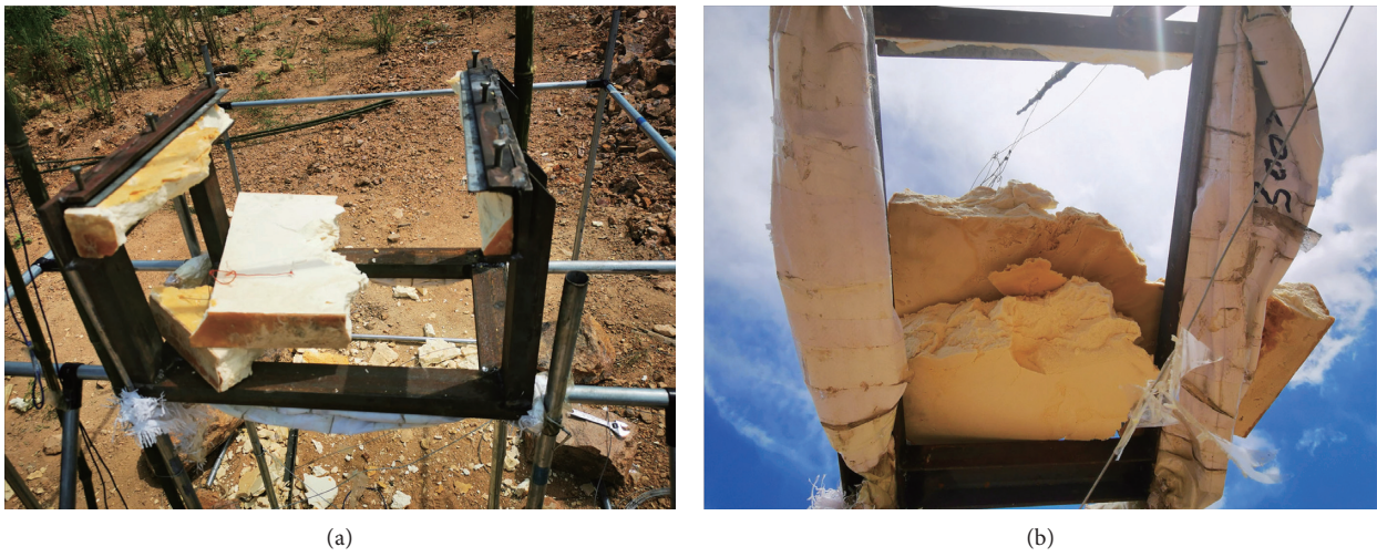
FIGURE 13: Test results of polymer slab B2 under 25 g explosive. (a) Top surface. (b) Bottom surface.
