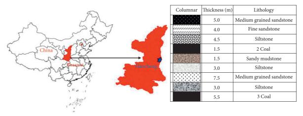
FIGURE 1: Location of the coal mine and its general stratigraphic column.
