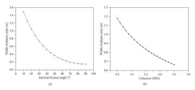
FIGURE 7: Relationship between width of plastic zone and internal friction angle and cohesion.
