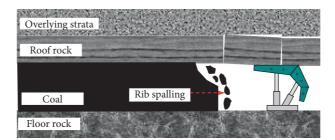
FIGURE 3: Schematic diagram of coal wall spalling.
