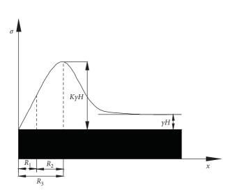
FIGURE 4: Coal body division and abutment pressure distribution.
