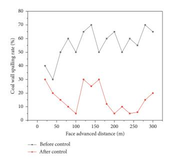
FIGURE 11: Comparison diagram of coal wall caving rate before and after treatment.
