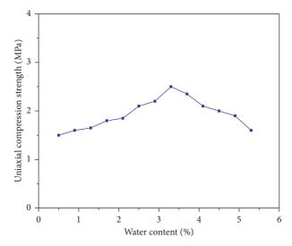
FIGURE 9: Variation trend chart of uniaxial compressive strength of soft coal with moisture content.
