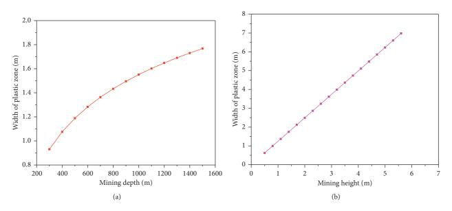
FIGURE 6: Relationship between width of plastic zone and mining depth and mining height.
