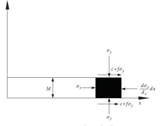
FIGURE 5: Force analysis of coal unit.
