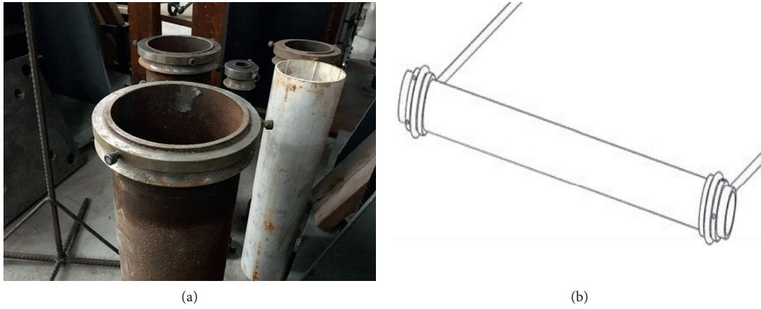
FIGURE 3: Connection between the steel strand and the test pipe. (a) Fixing device of the steel strand on the test pipe. (b) Schematic diagram of the fixed steel strand.
