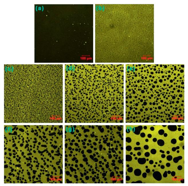
FIGURE 7: LSCM images of EA during curing at  $150^{\circ}$ C: 0 min (a), 3 min (b), 5 min (c), 10 min (d), 15 min (e), 20 min (f), 30 min (g), and 60 min (h) [108].
