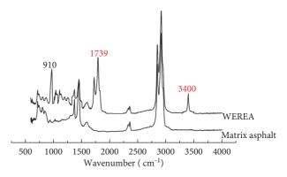
FIGURE 15: FTIR spectrum for WEA and asphalt [89].
