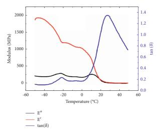
FIGURE 22: DMA properties versus temperature for EA [17].
