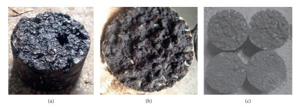
FIGURE 29: Interlaminar shear failure surface for EA-based prime coat (a, b) and common prime coat (c) [64].
