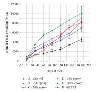
FIGURE 31: Resilient modulus for open-graded mixture with neat asphalt, SBA, and EA [18].
