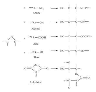
FIGURE 3: Reaction between epoxy and hardeners [11].
