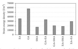
FIGURE 33: Strain energy density of asphalt mixtures [157]. Note: EA = epoxy asphalt; GA = Gussasphalt.
