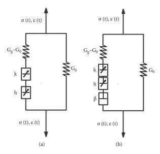
FIGURE 24: Huet-Sayegh model (a) and 2S2P1D model (b) [139].
