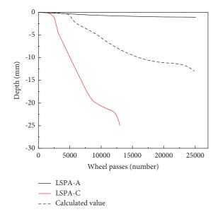
FIGURE 32: Depth profile for EAM [25]. Note: LSPA = blend of EA, LSP, and sand; calculated value = average depth of LSPA A and C.
