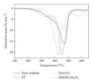
FIGURE 14: First derivative of the TGA curve [36].
