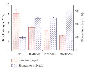
FIGURE 26: Tensile strength and elongation at break for ER and HMEA [7]. Note: ER = epoxy resin; HMEA = hot-mixed epoxy asphalt; 45, 50, and 55 = asphalt content by weight of HMEA binders.
