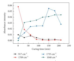
FIGURE 16: Evolution of epoxy group (917 cm<sup>-1</sup>), carbonyl acid (1709 cm<sup>-1</sup>), carbonyl ester (1735 cm<sup>-1</sup>), and carbonyl ether (1040 cm<sup>-1</sup>) [112].
