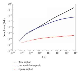
FIGURE 19: Creep behavior of binders at 40°C and 100 Pa [17].
