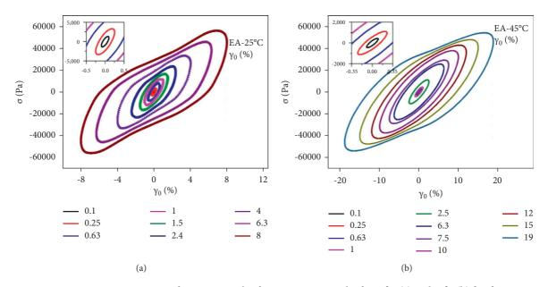
FIGURE 25: Lissajous curves for EA at angular frequency  $\omega = 6.3$  rad/s for 25°C (a) and 45°C (b) [141].
