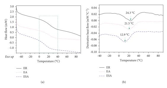
FIGURE 13: Nonisothermal DSC curves (a) and derivative of DSC curves of ER, EA, and ESA samples (b) [68]. Note: ER = epoxy resin; EA = epoxy asphalt; ESA = epoxy asphalt with SBS.
