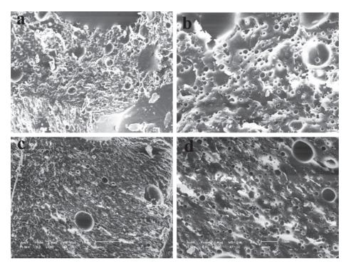
FIGURE 12: SEM micrographs of ER (a, b) and EA (c, d). (a, c) 600× and (b, d) 2000× [84].
