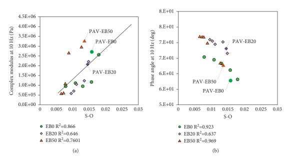
FIGURE 21: Relationship between sulfoxide compounds and complex modulus (a) and phase angle (b) during oxidative controlled curing [58].
