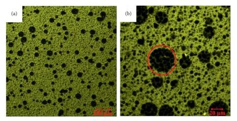
FIGURE 8: LSCM images of cured ESA: (a) ×100 and (b) ×400 [15].
