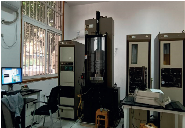
FIGURE 2: The MTS-815 system of Chongqing University.
