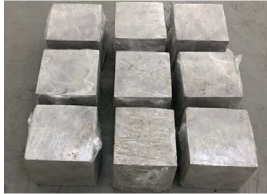
FIGURE 7: Partial processed sandstone specimens.
