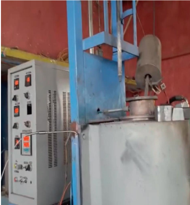
FIGURE 1: Stir casting machine.
