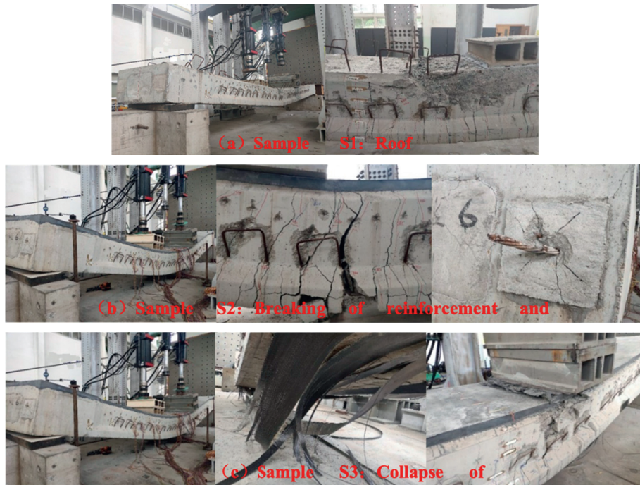
FIGURE 9: Failure of specimens S1, S2, and S3. (a) Sample S1: roof. (b) Sample S2: breaking of reinforcement. (c) Sample S3: collapse of UHPC.
