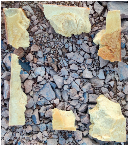
FIGURE 9: Test results of the polymer plate C3 under 8 g explosive.
