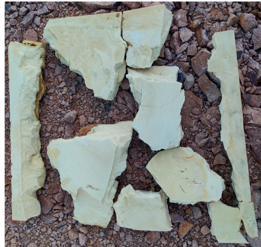
FIGURE 20: Test results of the polymer plate N3 under 10 g explosive.
