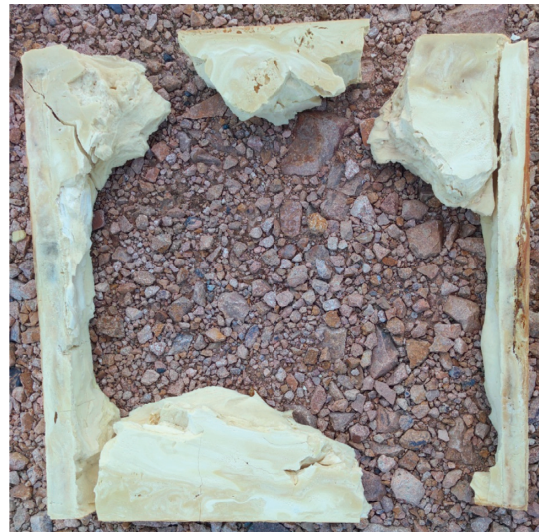
FIGURE 21: Test results of the polymer plate N4 under 20 g explosive.
