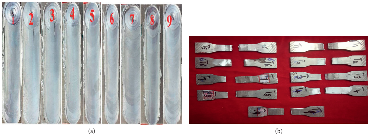
FIGURE 2: (a) Friction stir processed image and (b) prepared tensile specimens.
