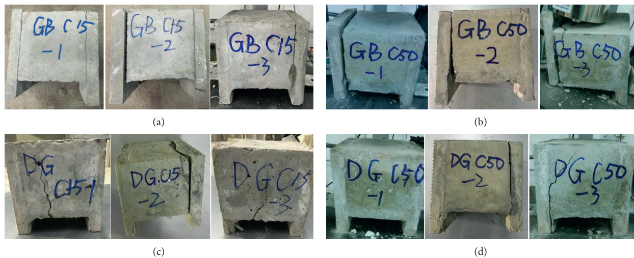
FIGURE 6: Failure characteristics of the composite samples after the shear test: (a) GB C15, (b) GB C50, (c) DG C15, and (d) DG C50.
