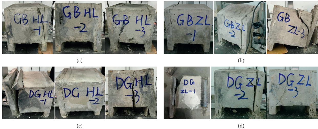
FIGURE 9: Shear fracture of cement plate and concrete composite specimens with different ribs: (a) GB HL, (b) GB ZL, (c) DG HL, and (d) DG ZL.
