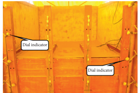
FIGURE 6: The real layout of the dial indicator.
